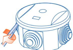
Opening the round box with IP44 protection is shown on Fig.1
